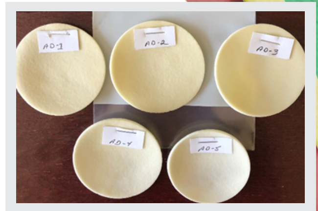
Hexane extracts the DIDP causing significant shrinkage and loss of flexibility.
